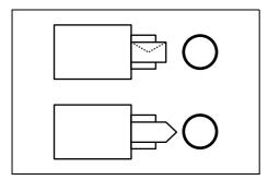
**3** For landscape form envelopes, close the flap. Insert the envelope all the way along the width guides, keeping the printing side face-up and the flap closed.
